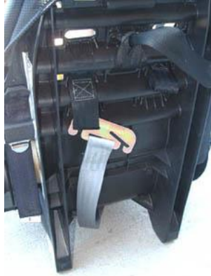
Straps Detach via Rear Bracket
